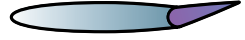
MOVING THE RUDDER TO THE RIGHT FORCES THE TAIL TO THE LEFT.
